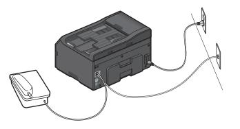
**2** Remove the protective plug from the import of the printer, and then connect the telephone to the port.
